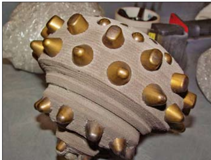
The carbide inserts of this 8-in. OD drillbit were clad with a dissimilar metal to protect the wear surfaces and extend service life (Fig. 4, photo from Laser Cladding Services Ltd.).
