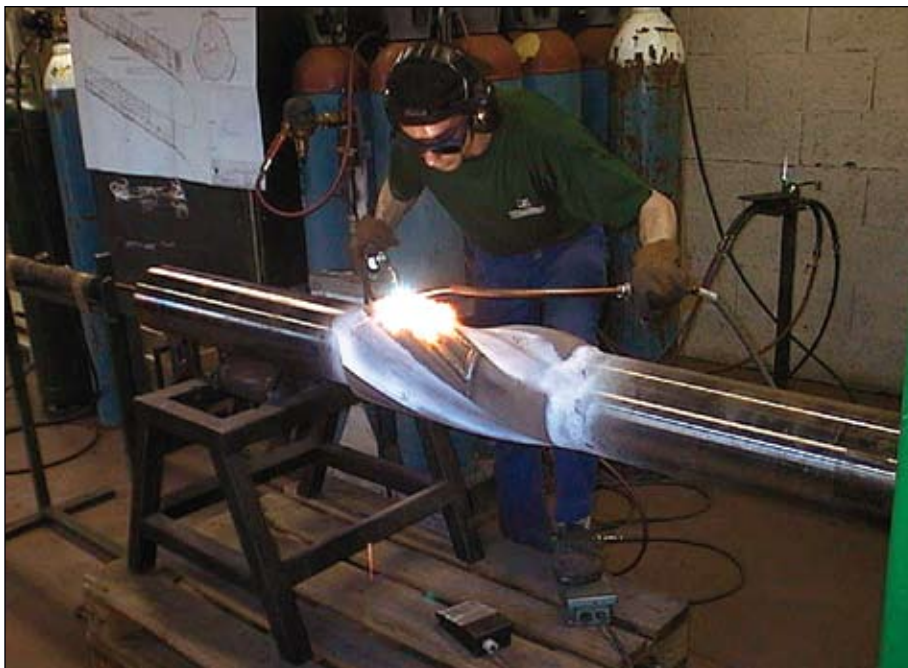
Using an oxyacetylene torch, a welder applies a tungsten carbide-nickel alloy hard facing material in the form of a continuous, flexible rod or "rope" (Fig. 3; photo from Technogenia).
